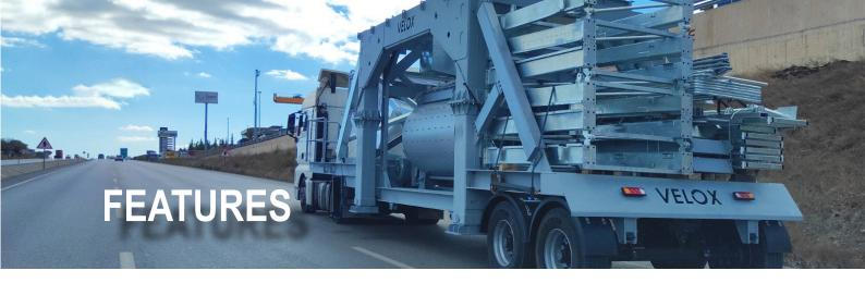
VELOX mobile plants have the capacity from 60m3/hr up to 120m3/hr. As the contractor companies needs to move their plants frequently, mobile plants are the ones which supply concrete where ever they needed to. Whenever there is a space limitations, mobility and fast set up are concerned, IME mobile plants are the optimal solution with high European standarts.
